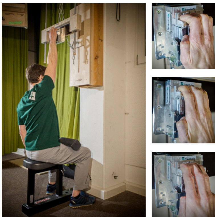
Figure 1: The structure with variable height adjustment for the force measuring device to guarantee optimal shoulder centering is shown in the left part of the figure. The body can be braced against the device with the help of a bar above the upper legs. In the right part of the figure the finger positions are shown. From top to bottom half crimp with four fingers (HC4), slope handgrip with four fingers (SG4) and slope handgrip with three fingers (SG3).
