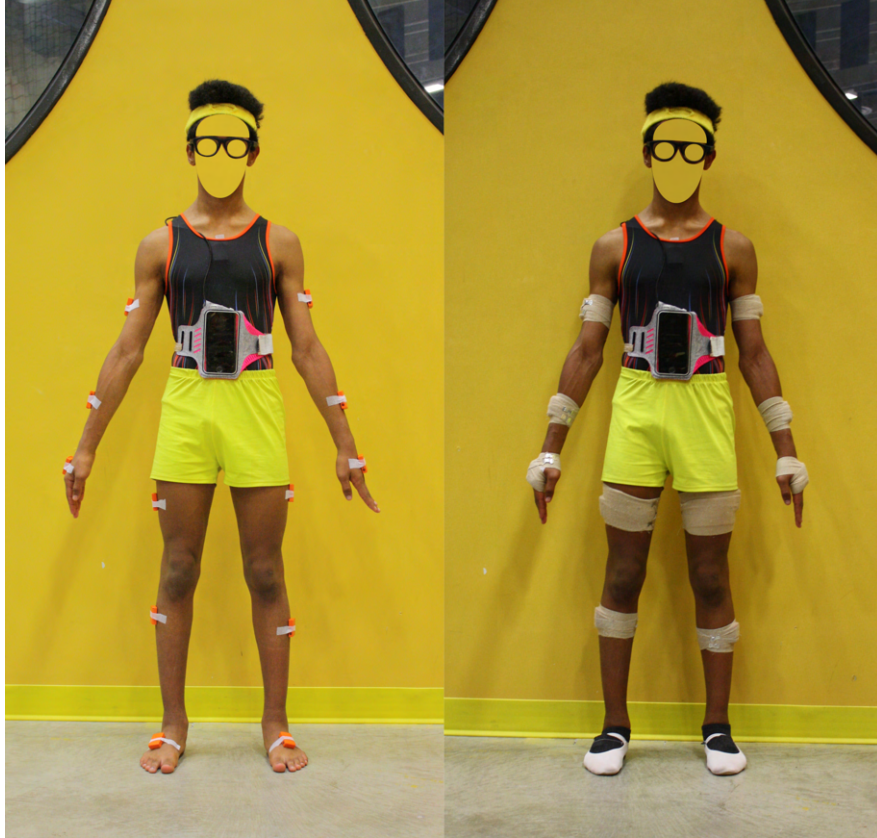
Figure 2. Illustration of a trampolinist equipped with the 17 IMUs and the wearable eye tracker (left). The IMUs were covered with elastic bands to fix them on the athlete's segments (right).
