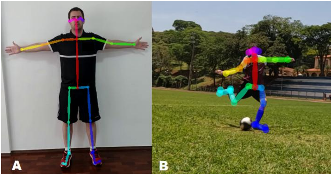
Figure 2: A: OpenPose detection demonstration. B: OpenPose applied to kicking task.
