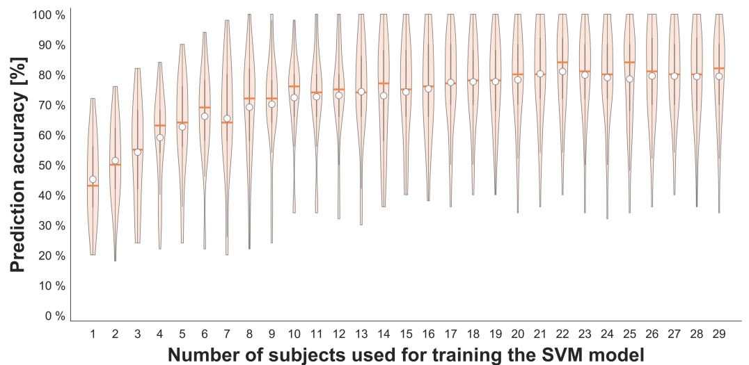
Figure 4. Performance evaluation of the machine learning models trained for footwear classification with different number of subjects used for training the support vector machine (SVM) models. The prediction accuracy was obtained using a leave-subject-out cross-validation configuration shown as violin plots with median (solid line) and mean (white dot). Created using the MATLAB code provided by Bechtold et al. (2022). 34
