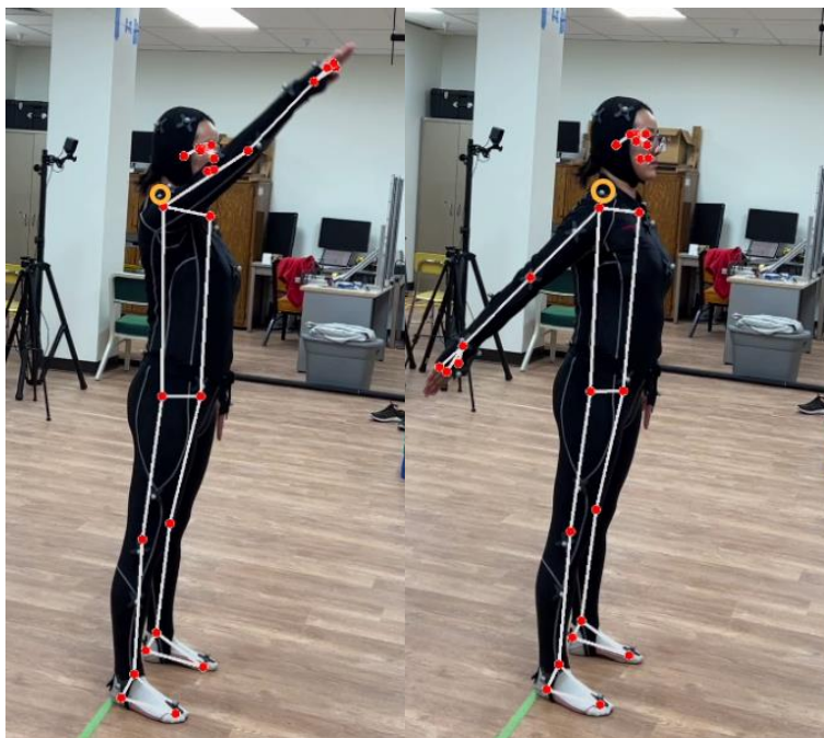
Figure 4. A participant performing the shoulder flexion (left) and extension (right) movements. The orange circle highlights the locations of the OptiTrack markers.
